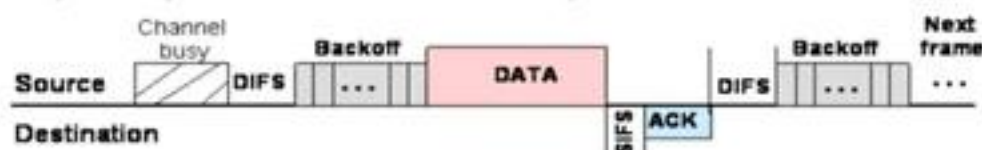
Fig. 1: Basic Operation of IEEE 802.11 DCF
