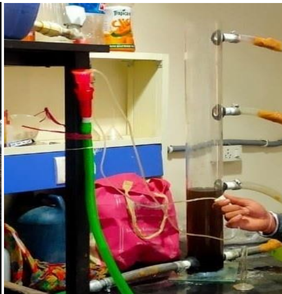
Figure-3: UASB Reactor
